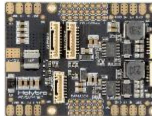
Connect to the Power Management Board using the 6-wire cable to direct power from your lithium polymer (LiPo) battery to the autopilot.
