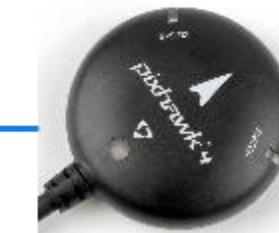
Connect the provided GPS module (with integrated compass, safety switch and buzzer) to provide the autopilot with positioning data during flight.
