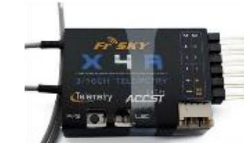
Connect PPM, DSM or SBUS Radio Control receiver to provide the autopilot with RC input in manual and assisted flight modes.
